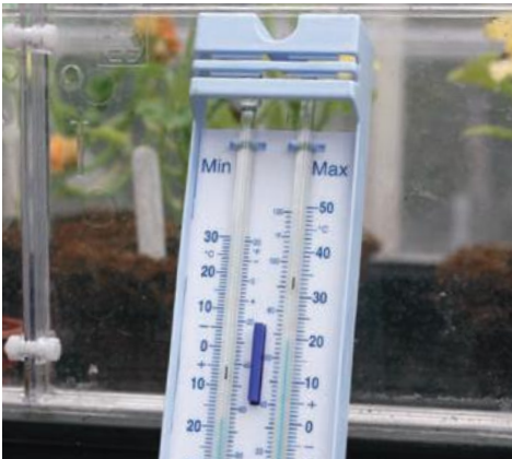
A maximum-minimum thermometer will record daily fluctuations in temperature
